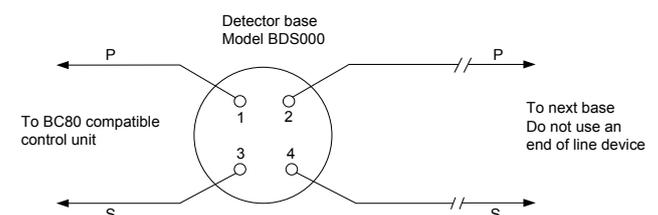
Figure 2 Installation and wiring diagram
