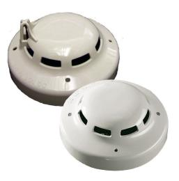
The FAP-325 Series Analog Smoke and Smoke/Heat Detectors are addressable devices used in the analog polling circuit. They detect fast-flaming fires and dense smoke typically given off by plastic, foam, paper, wood, and other materials that tend to smolder.
