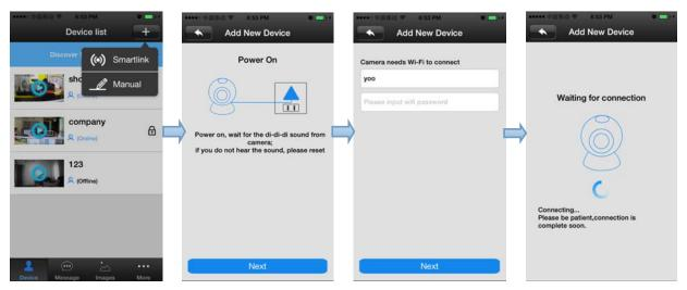
3) Add device manually: in the device interface of the Yoosee software, click the "+", input ID and password is ok.
