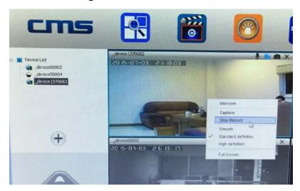
2) playback: this device can playback the video from computer, open the CMS software, click on the replay button, choose "playback", user can find the playback files according to the date, then play it directly.
