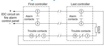
End-of-line resistor required on last device for circuit supervision. Use resistor value specified by the fire alarm panel manufacturer.
