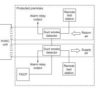
building. It is typically used to detect smoke in the supply side of the HVAC system but can provide supervision of the return side as well.
