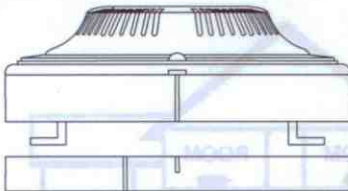
Figure 4: Alignment of detector head and its base.
