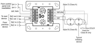
The FX-2WIRE can be set for Class B or Class A operation using the slide switch located on the front of the module.
