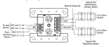
contact initiating devices. When the NO input contact of an initiating device is closed, a supervisory signal is sent to the control panel and the supervisory condition is not latched at the module.
