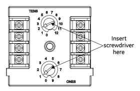
**Example:** device address 21, set TENS rotary switch to 2 and set the ONES rotary switch to 1.
