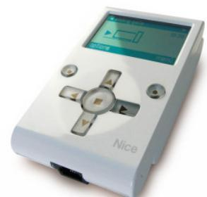
O-View programmer is used by the installer to advance features and fine tune motor functions.
