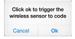
Click "confirm", and trigger the alarm you will learn at the same time(take the door sensor as example, separate the door sensor will trigger the alarm).if match code successfully, the words will be turn blue from gray, and will pop-up :learn successfully".
