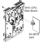
Note: All networked panels must have a 3X-NET8 network card installed.
