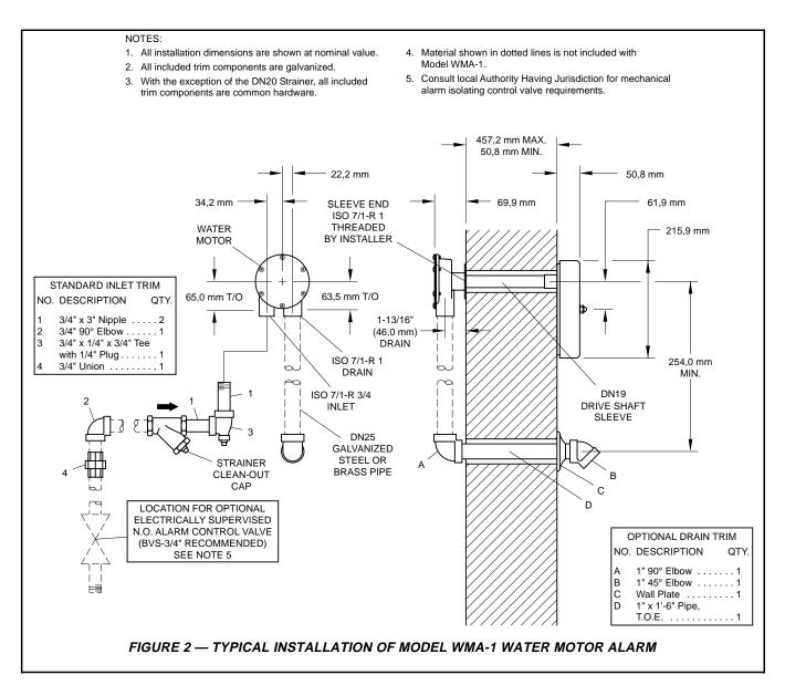
**Step 6.** Tighten the ISO threaded end of the Sleeve into the Body hand tight plus 1/8 turn.
