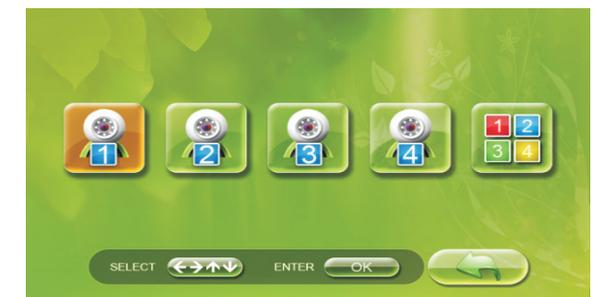
Monitoring channel has 1/2/3/4 / and four split screen. When only one outdoor unit, select to choose channel. press button to confirm. Can choose channel when you have more wireless outdoor unit. When required for monitoring a plurality of screens, can use four split screen while monitoring.
