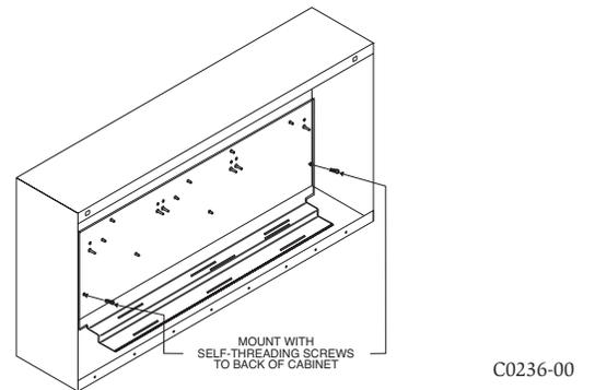
The BB-XP cabinet comes with the chassis already installed, so no mounting is necessary.
