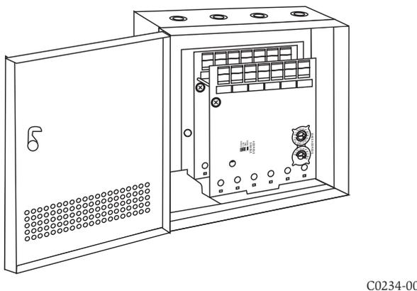
The front XP6-C module positions of each chassis are offset below the rear XP6-C module positions so that all of the status indicators are visible.
