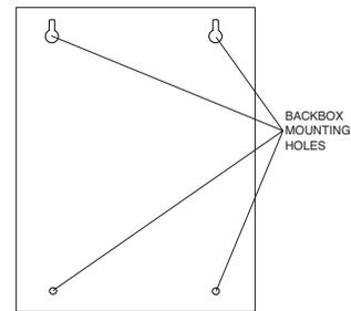
**FIGURE 4: MOUNTING THE CHS-6 CHASSIS**
